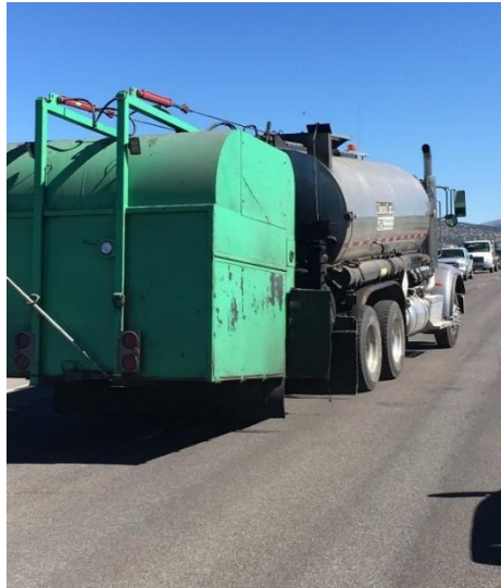
Figure 5.2. Photo. Asphalt binder distributor with emissions capture apparatus.
