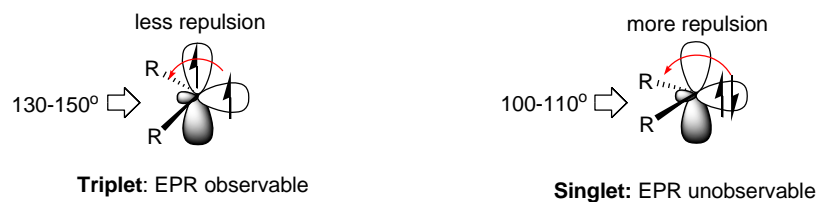
Figure 2-3 Bond angle differences in triplet and singlet carbenes
