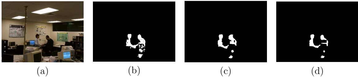
Figure 4.1: Rapidly fluctuating background: (a) Handshake video sequence. Detected foreground regions using (b) AKDE. (c) RM. (d) SVDDM.
